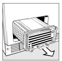
Pull out the heat exchanger
